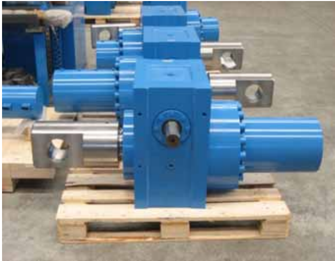
Screw jack with incorporated load cell
