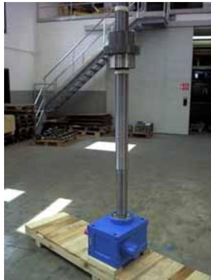
Screw jack with incorporated load cell
